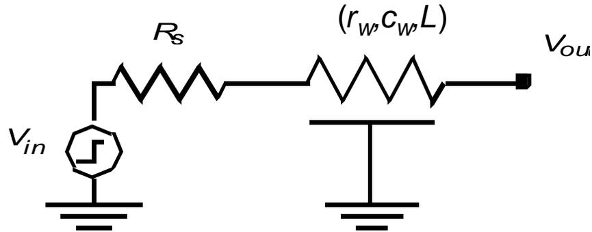
$$\tau_D = R_s C_w + \frac{R_w C_w}{2} = R_s C_w + 0.5 r_w c_w L^2$$
