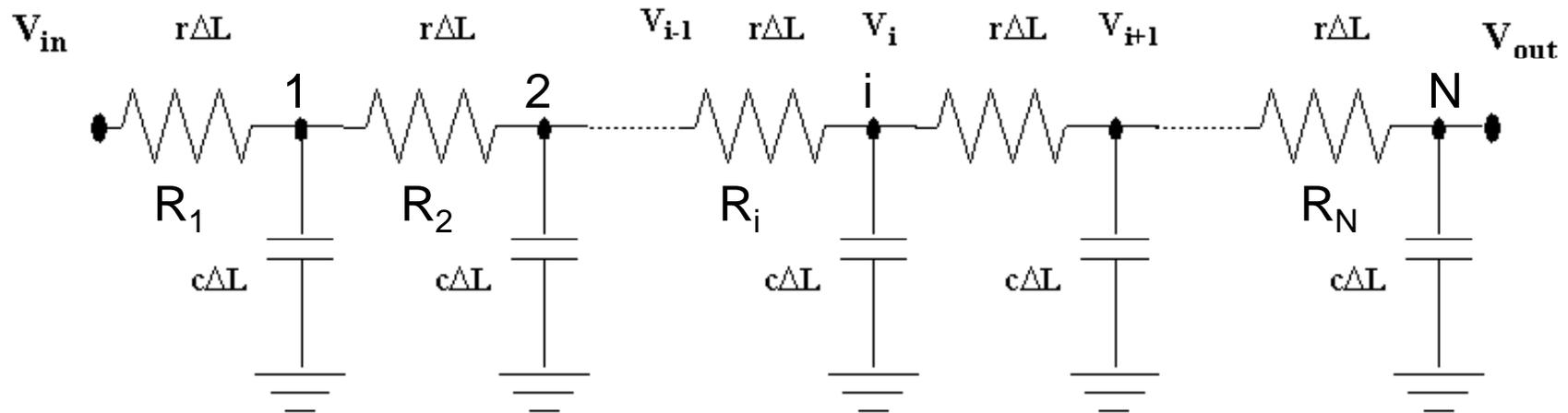
Elmore delay of node  $i$ :  $\tau_i = R_1 C_1 + (R_1 + R_2) C_2 + \dots + (R_1 + R_2 + \dots + R_i) C_i$
