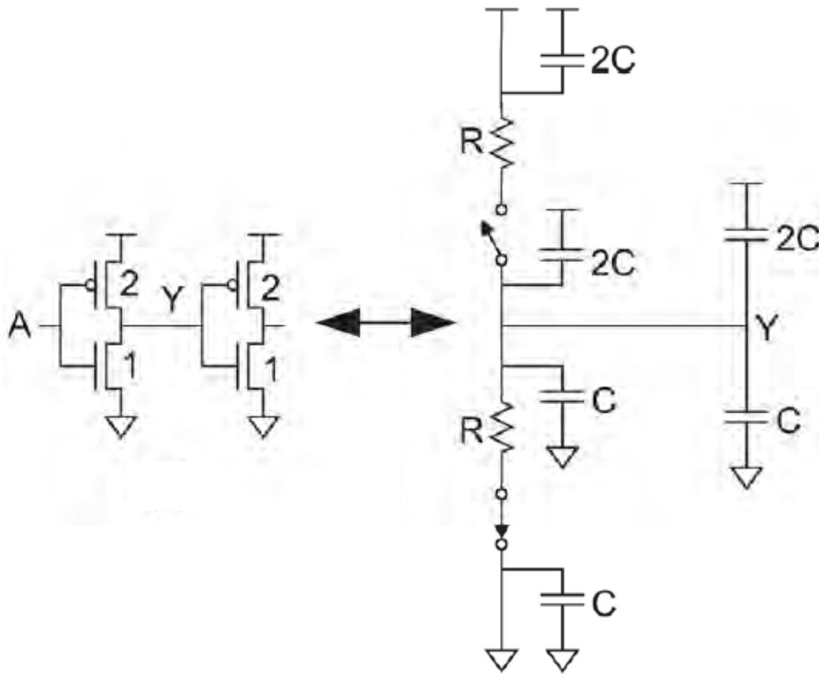
Estimation of delay of a fanout-of-1 inverter.
