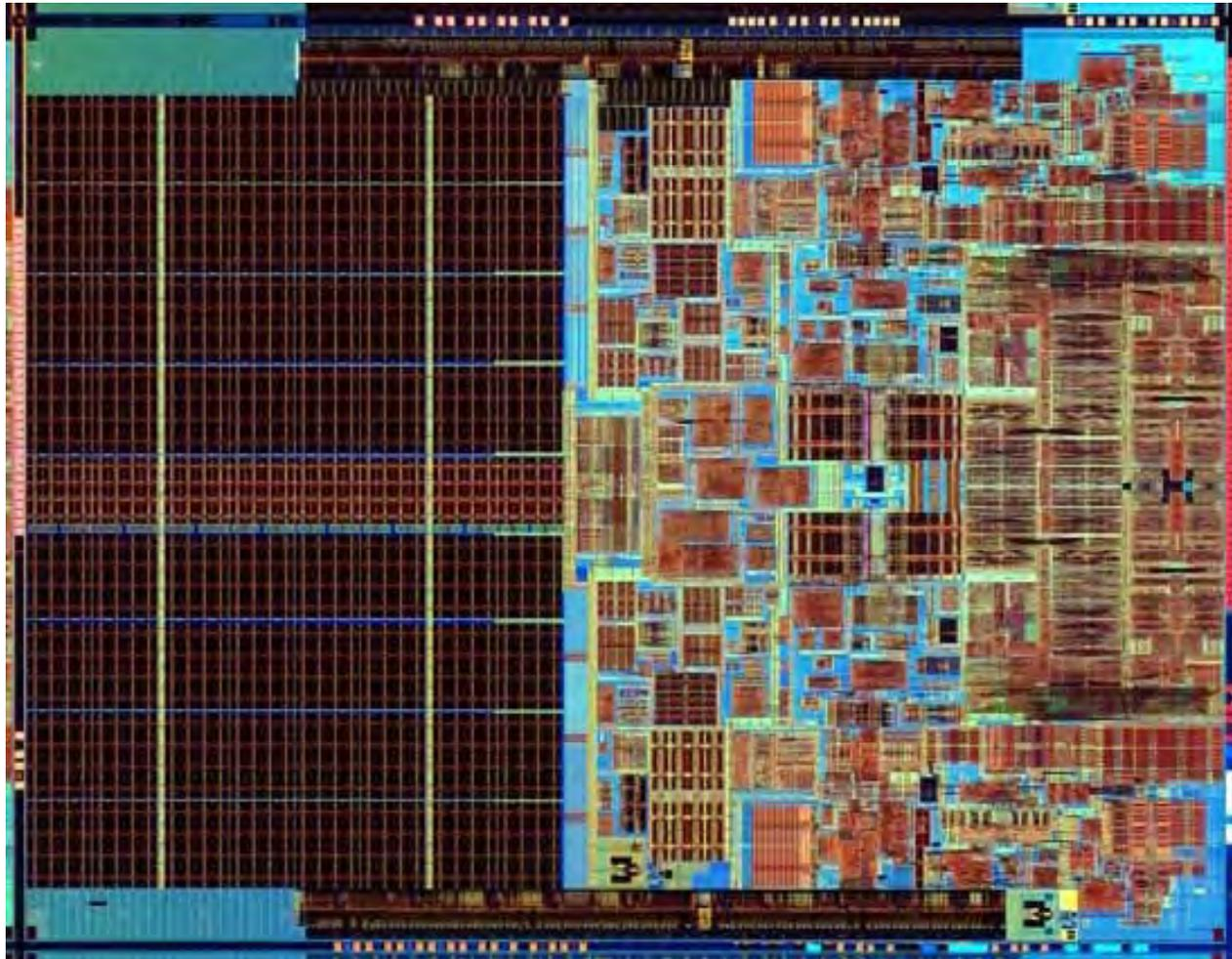
Core 2 Duo T5000/T7000 series mobile processors, called Penryn uses 800M of 45 nanometer devices (2007).
