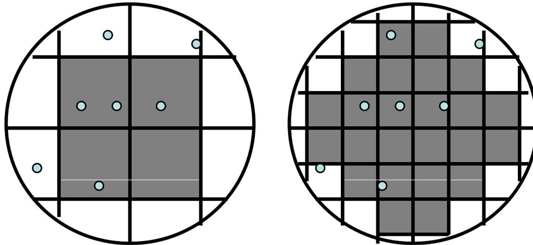
$$\text{die yield} = \left( 1 + \frac{\text{defects per unit area} \times \text{die area}}{\alpha} \right)^{-\alpha}$$
