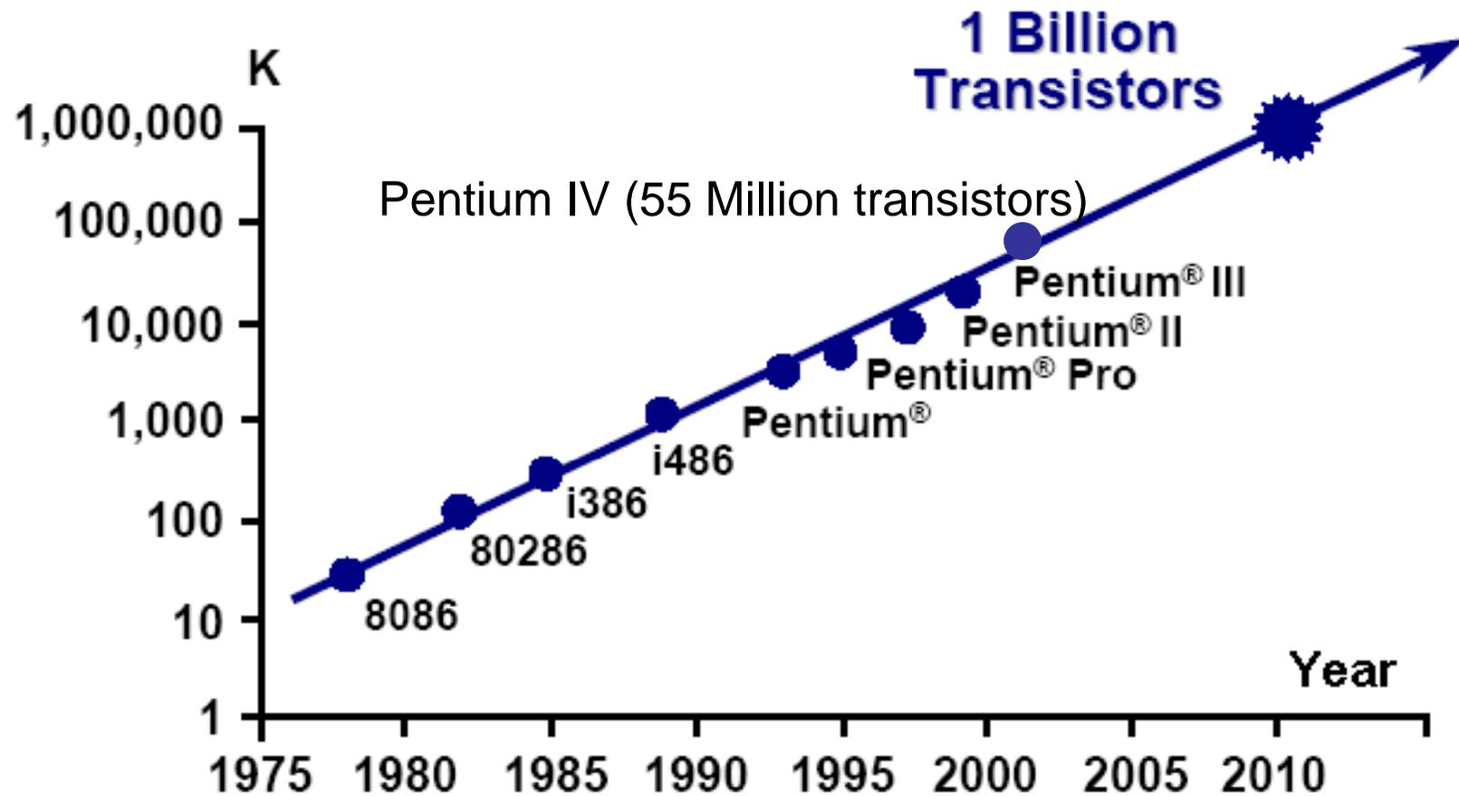
**Transistors on Lead Microprocessors double every 2 years**
