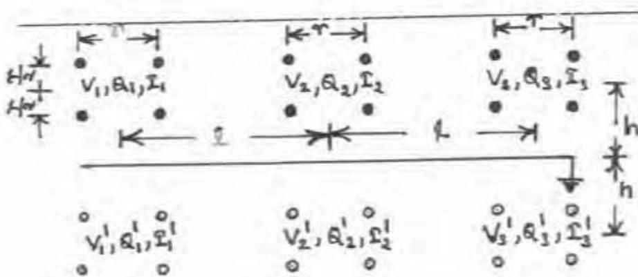
FIG1. SCHEMATIC REPRESENTATION OF A THREE PHASE EHV SYSTEM WITH IMAGE ARRAYS.
