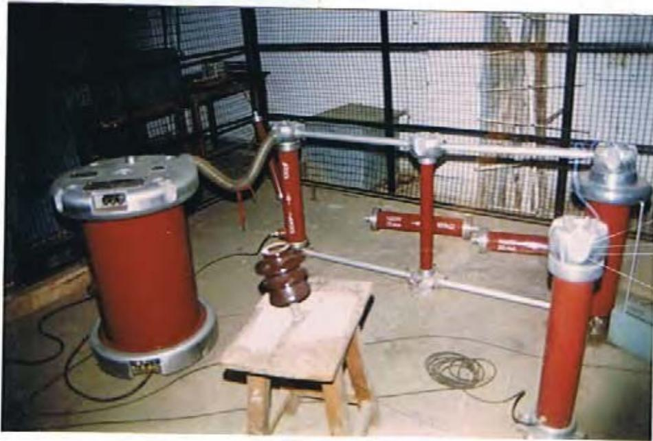
FIG.1. EXPERIMENTAL SET UP FOR AC CORONA
