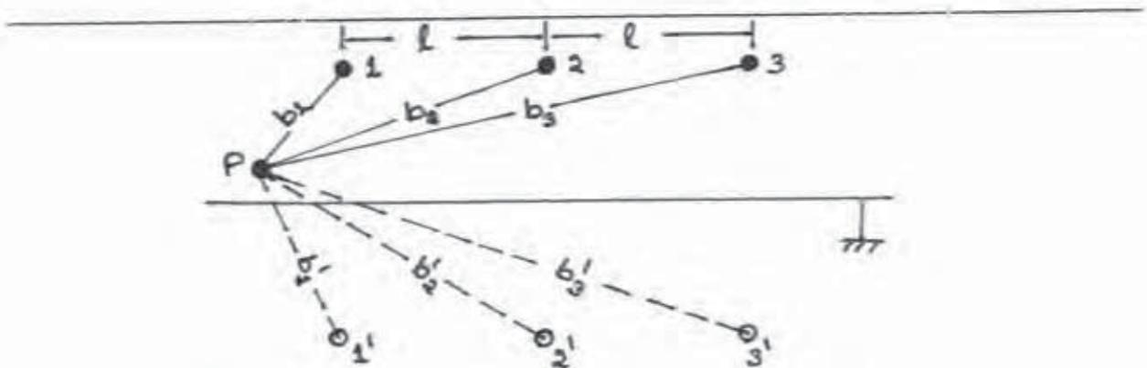
FIG.3. THREE PHASE SYSTEM WITH THE ARRAY OF CONDUCTORS Banded TOGETHER IN THEIR RESPECTIVE PHASES.
