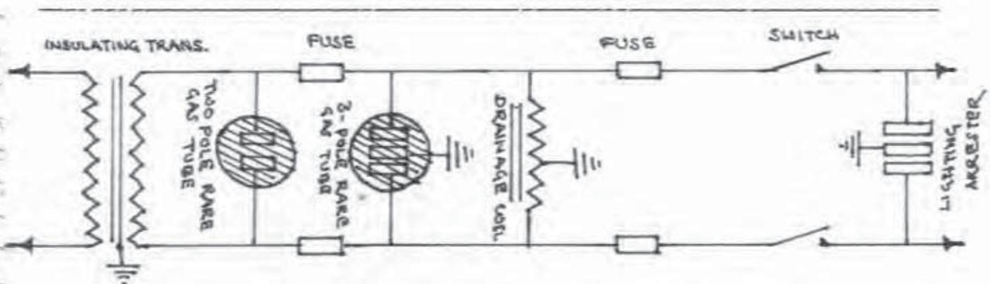
FIG.6. PROTECTIVE SYSTEM FOR COMMUNICATION CIRCUIT
