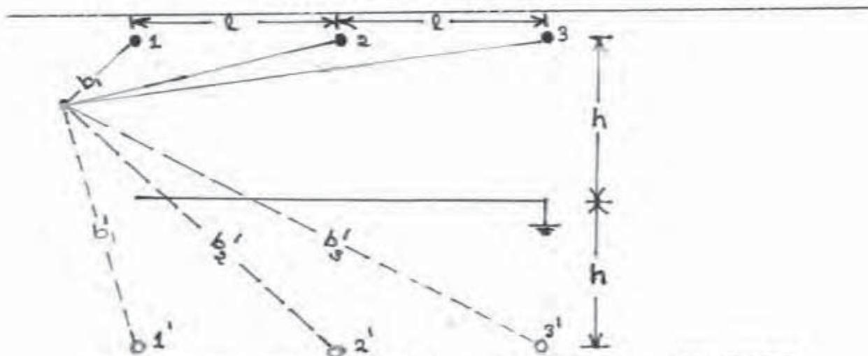
FIG.2 THREE-PHASE SYSTEM WITH THE ARRAY OF CONDUCTORS BUNDLED TOGETHER IN THEIR RESPECTIVE PHASES.
