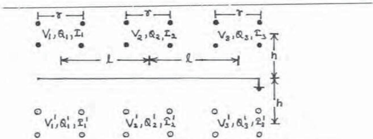
FIG.1 SCHEMATIC REPRESENTATION OF A THREE-PHASE EHV SYSTEM WITH IMAGE ARRAYS.
