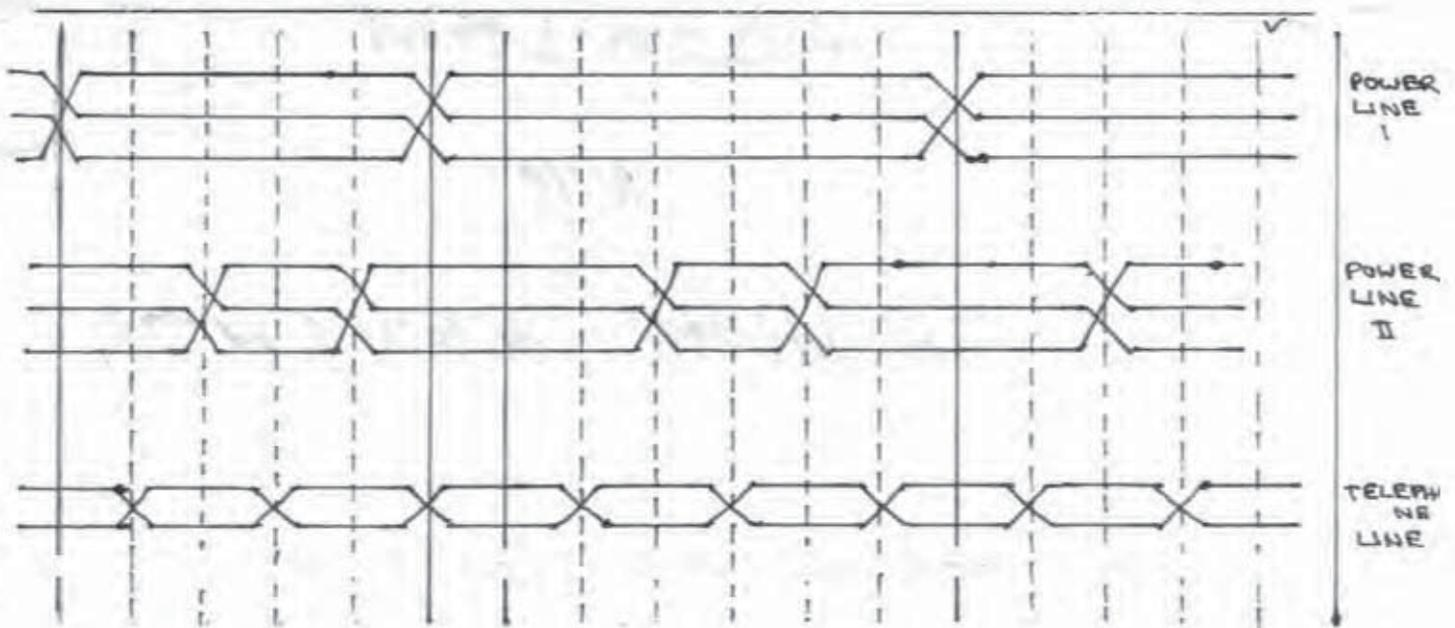
FIG.4 TRANSPOSITION SCHEME FOR TWO POWER LINES & A TELEPHONE LINE
