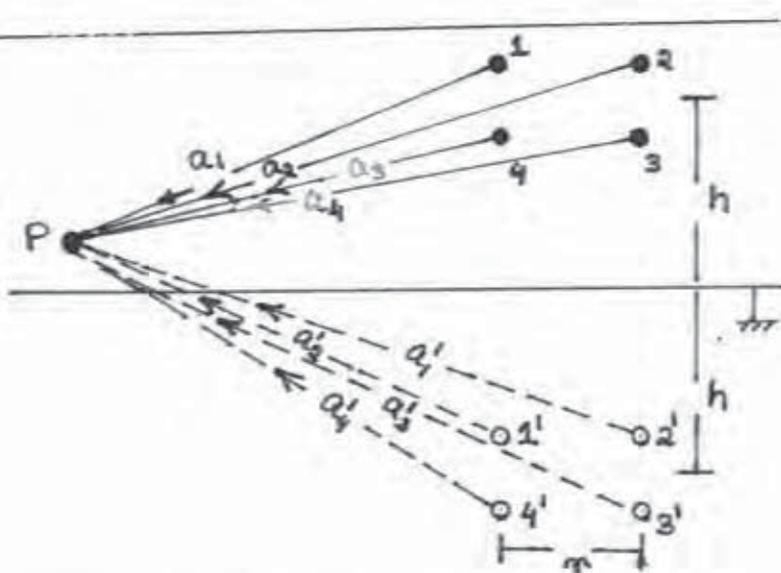
FIG.2. AN ARRAY OF FOUR CONDUCTORS & ITS IMAGE
