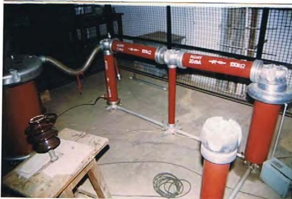
FIG.2. EXPERIMENTAL SET UP FOR DC CORONA
