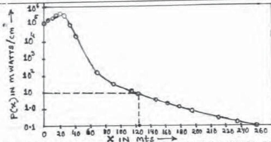
FIG.4. VARIATION OF GROUND LEVEL ENERGY FLUX IN THE LATERAL DIRECTION.
