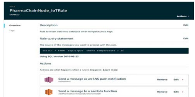
Fig. 10b: IoT Custom Rule to Check Abnormal Temperatures
