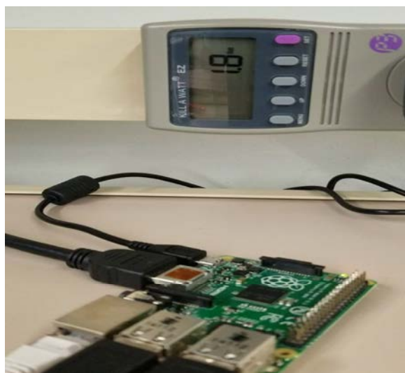
Figure 14. Electric Meter Setup for Measuring Power Consumption in Implemented EasyChain
