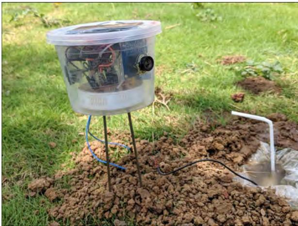
(a) Prototype setup with no irrigation.
