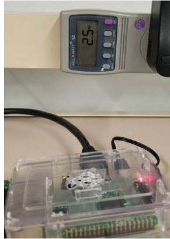
(b) Maximum power consumption of Raspberry Pi 2 Model B+
