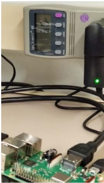
(a) Maximum power consumption of Raspberry Pi 3 Model B+
