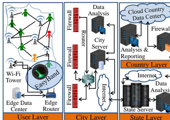
Fig. 3: EasyBand in Healthcare of Cyber-Physical System (H-CPS) of the City, State, and Nation.
