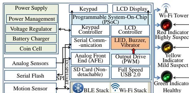
Fig. 4: The Architecture of Proposed EasyBand.
