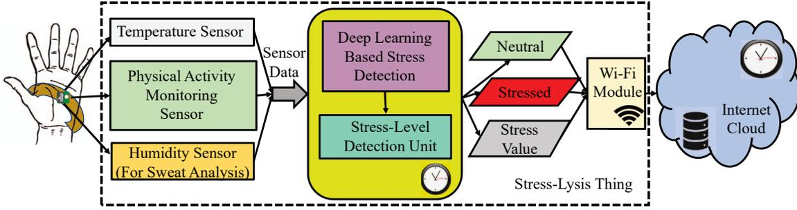
Fig. 3. The proposed architecture of the Stress-Lysis system.
