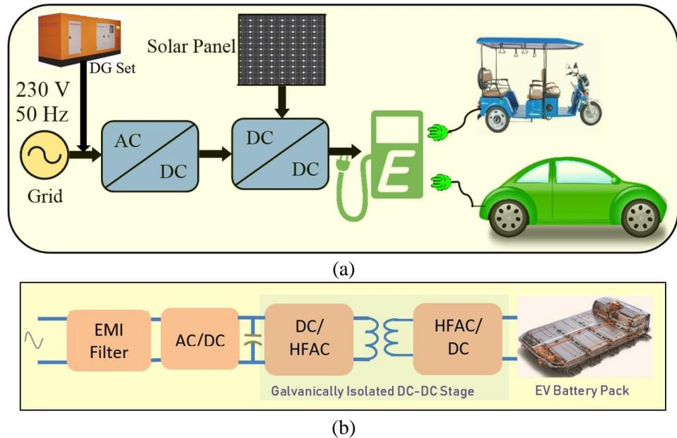
FIGURE 6. (a) Mix-energy source EV charging and (b) Typical on-board EV charger architecture.
