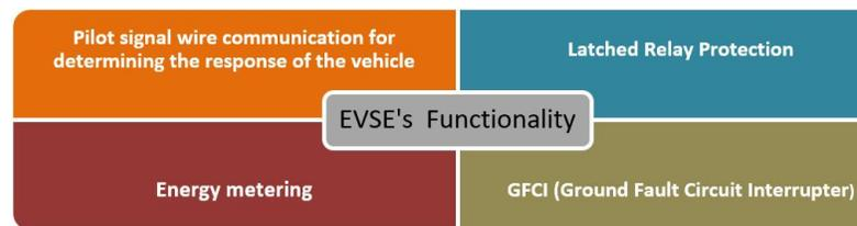
FIGURE 4. Functions of EVSE.
