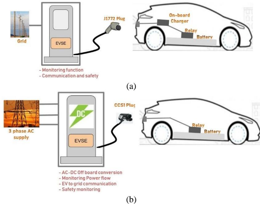
FIGURE 3. Different types of charging technology: (a) Components of AC charging station: uses on-board charger inside an EV (b) Components of DC charging station: directly charges the EV battery.
