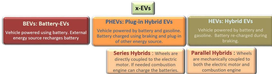
FIGURE 1. A broad classification of different EVs.
