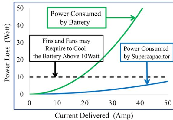
FIGURE 2. Supercapacitor versus Battery.
