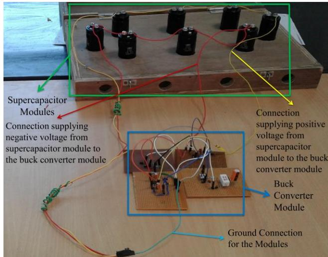
FIGURE 3. Prototyping of supercapacitor powered battery-less buck converter.
