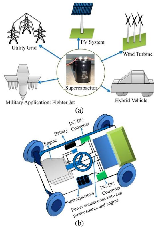
FIGURE 1. (a) Diverse application of supercapacitors. (b) A super capacitor based hybrid vehicle.
