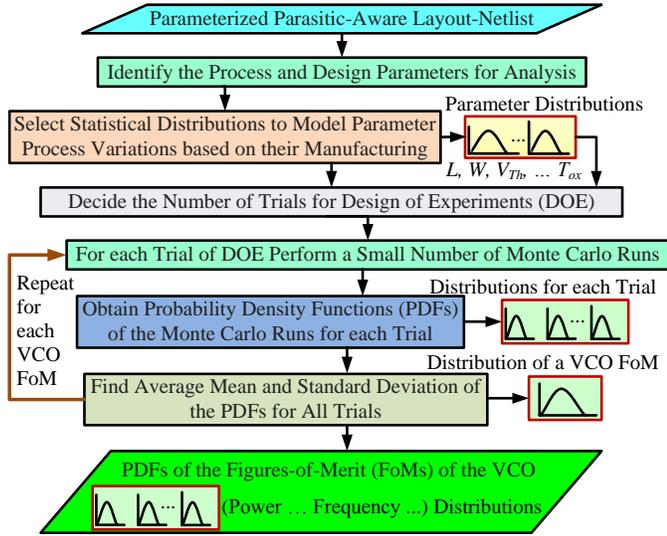
Fig. 4. Proposed Design-of-Experiment assisted Monte Carlo (DOE-MC) for fast process variation analysis.
