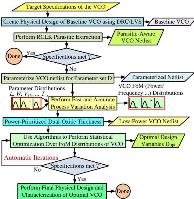
Fig. 3. The proposed novel process variation aware design flow which obtains an optimal physical design of a VCO in a single manual iteration compared to multiple manual iterations of a standard flow.
