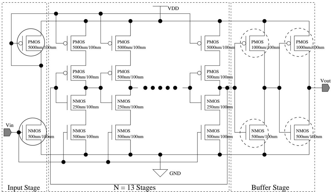
Fig. 6. Logical design of a current-starved VCO. The VCO has 13 stages. The transistor sizes are provided in Section VI. The solid circled transistors consume 48% of the total average power while the dashed circled transistors consume 11.5% of the total average power as discussed in Section VII.
