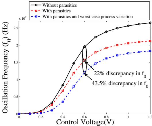
Fig. 1. Frequency-voltage characteristic degrades when the parasitic-extracted physical design is subjected to worst-case process variation.
