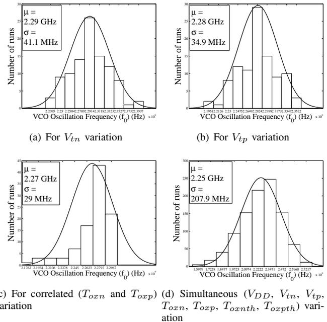
Fig. 10. Statistical process variation analysis of the optimal VCO.
