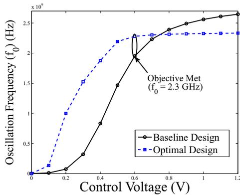
Fig. 11. Frequency-voltage characteristics of the optimal VCO.
