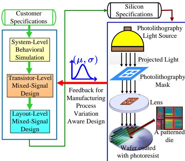
Fig. 2. Incorporating manufacturing process variation in early design to enhance chip yield.
