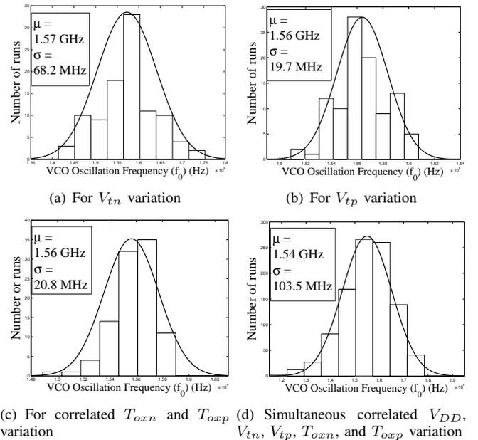
Fig. 8. Statistical process variation analysis of the baseline VCO for the individual variation of  $V_{tn}$  and  $V_{tp}$ , correlated  $T_{ox}$  variation, simultaneous correlated  $V_{DD}, V_{tn}, V_{tp}, T_{oxn}$ , and  $T_{oxp}$  variation. The distribution of  $f_0$  is observed to be Gaussian in all cases.
