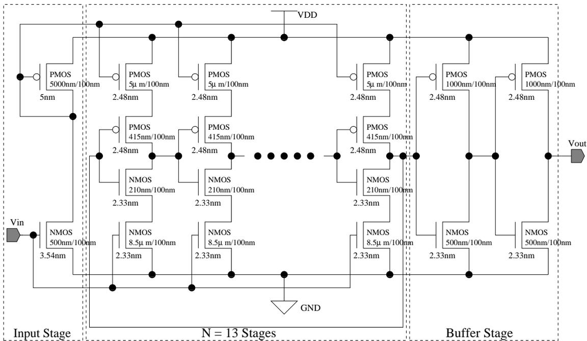
Fig. 9. Final widths and gate-oxide thicknesses of transistors of the process variation optimal VCO.
