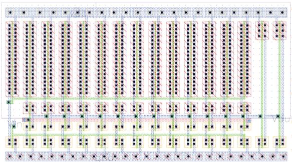
Fig. 7. Physical design of the 90nm CMOS based baseline VCO. The area of the VCO is  $228.43 \mu\text{m}^2$ .
