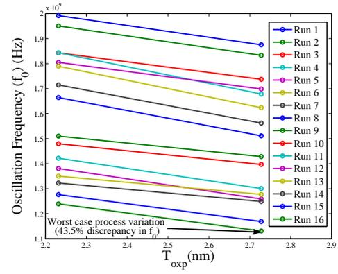
Fig. 5. Effect of parameter variation on oscillation frequency ( $f_0$ ) of the VCO for the parameter  $T_{oxp}$ .
