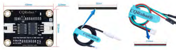
Fig. 3: Necessary Components for TDS Measurement
