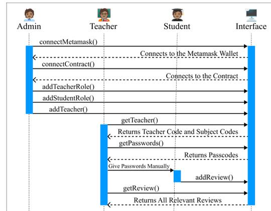
Fig. 3. Sequence Diagram of Proposed AcadChain implementation
