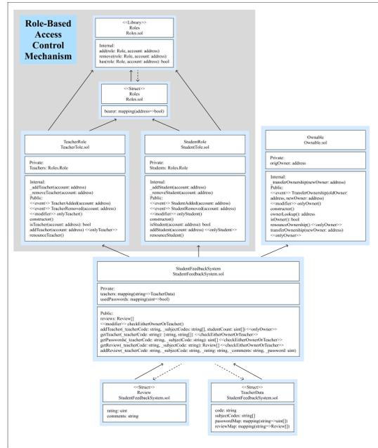
Fig. 5. Class Diagram of Proposed AcadChain solution
