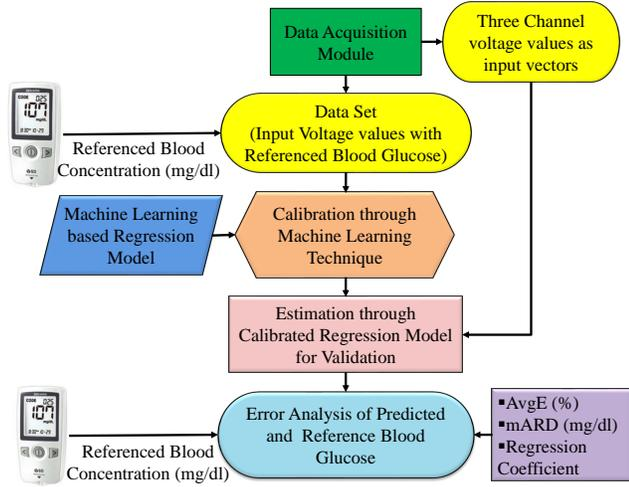
Fig. 3: Calibration and Validation of proposed iGLU device.
