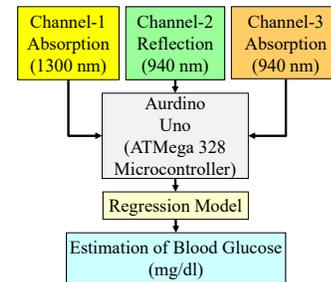
Fig. 2: Processing steps for the Proposed iGLU.
