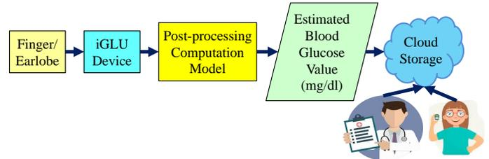
Fig. 1: Non-invasive glucose level measurement using iGLU in IoMT.
