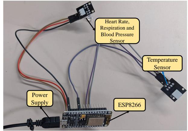
Fig. 7. Hardware Implementation of Smart-Steering
