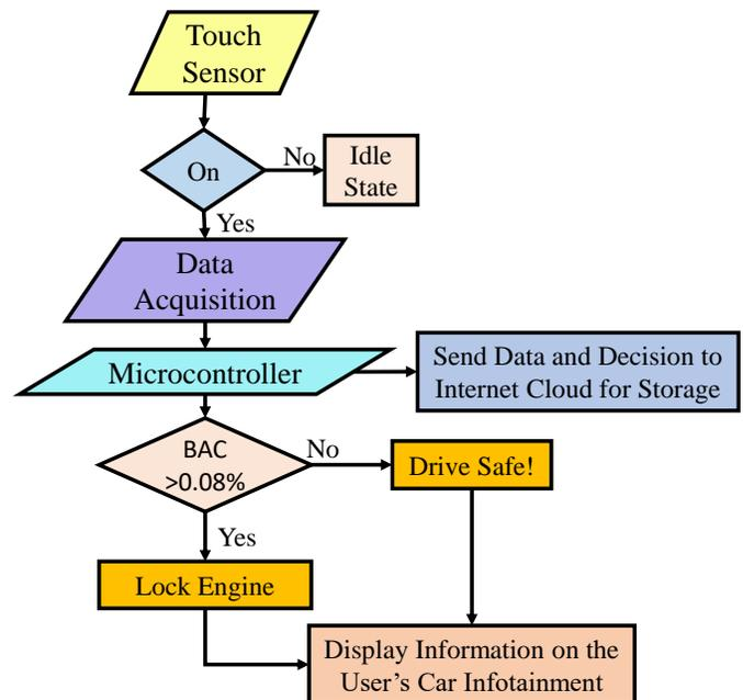
Fig. 5. Design Flow of Smart-Steering
