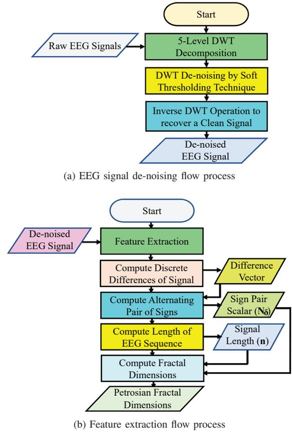
Fig. 4: Real-time seizure detection flow process in segments.
