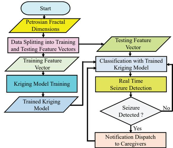
Fig. 5: Model training and seizure detection flow process
