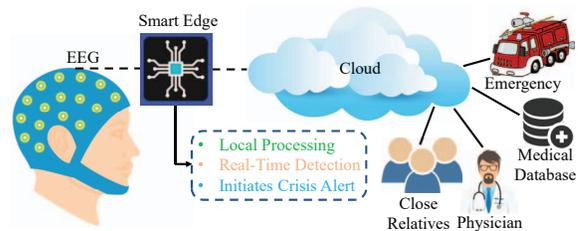
Fig. 3: Proposed edge computing model for seizure detection
