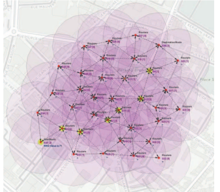
Fig. 5. A* algorithm modeled in CupCarbon
