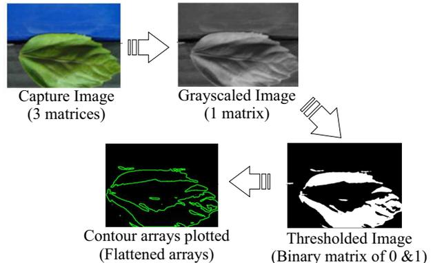
Fig. 2. The conceptual block diagram of estimating leaf contour using image analysis
