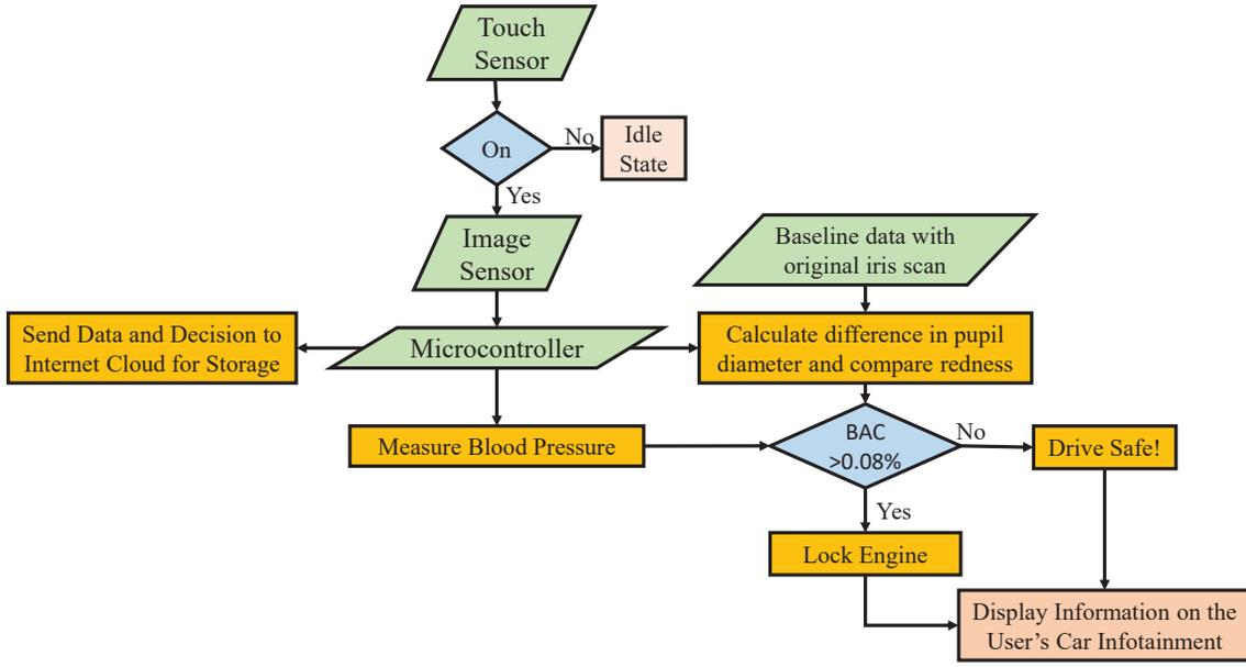
Fig. 5: Working Principle of Donot-DUEye
