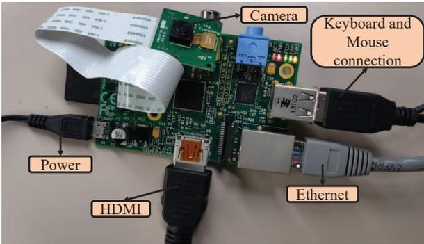
Fig. 8: Raspberry Pi Platform for Donot-DUEye System
