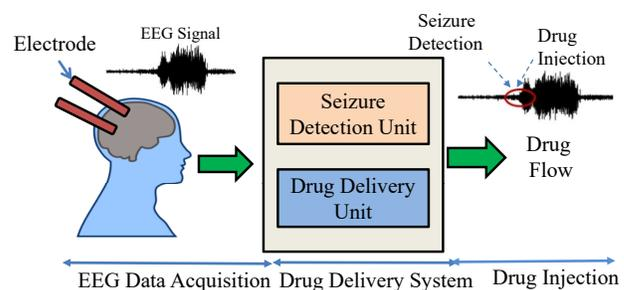
Fig. 1: Block Diagram of the Drug Delivery System (DDS).
