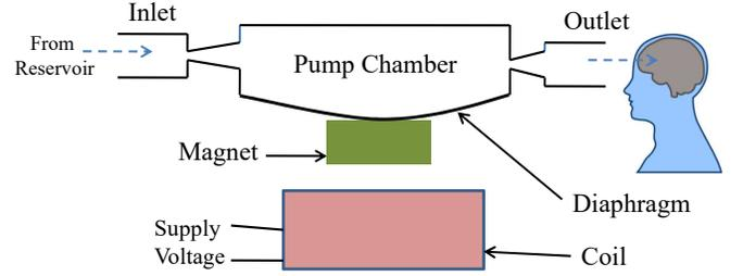
Fig. 5: Electromagnetic Actuated Valveless Micropump (EAVM).
