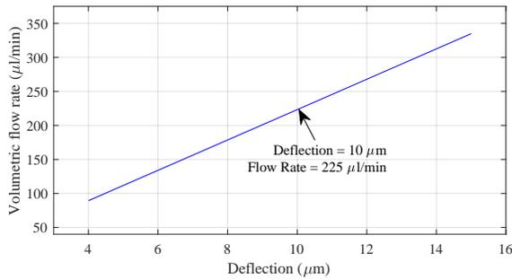
Fig. 7: Volumetric Flow rate as a Function of Membrane Deflection.
