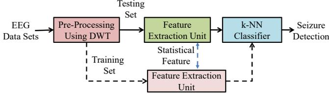
Fig. 4: Architecture of the Proposed Seizure Detection Unit.
