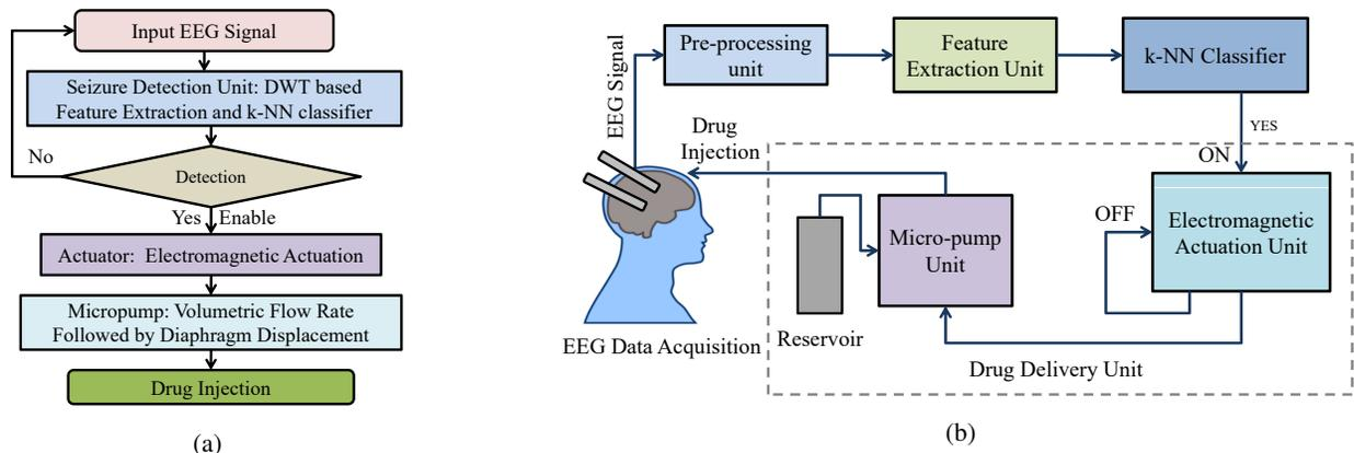
Fig. 3: Proposed Drug Delivery System (a) Flowchart (b) Architecture.
