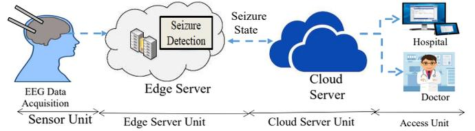
Fig. 2: Architecture of the proposed system in the edge-IoT perspective.
