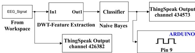
Fig. 4: Simulink and Arduino based prototyping of the proposed system.
