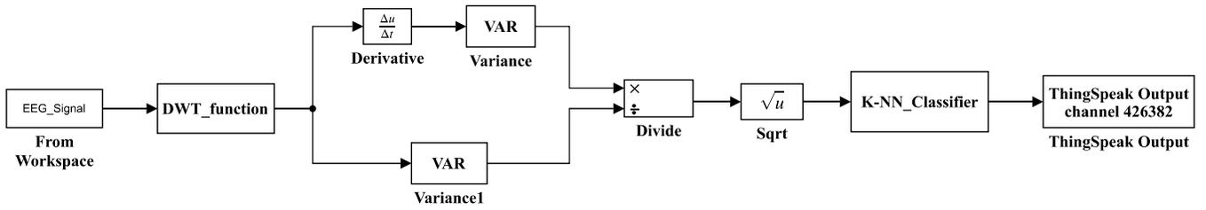
Fig. 4: Simulink<sup>®</sup> model of the proposed system.
