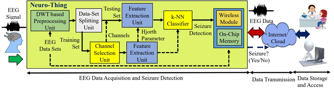
Fig. 2: Block diagram of the proposed novel IoMT-enabled seizure detector architecture.
