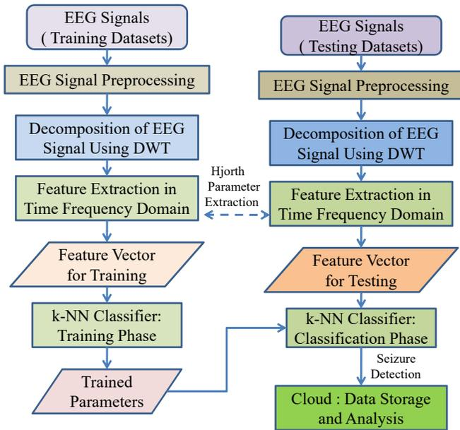
Fig. 3: Flowchart of the proposed novel fast and accurate seizure detection algorithm.
