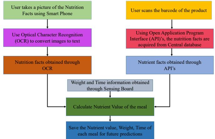
Fig. 2: Flow chart of data acquisition involved in the nutrition monitoring system.
