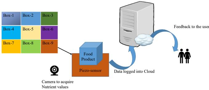
Fig. 1: Overview of IoT based sensor system for Smart-Log.
