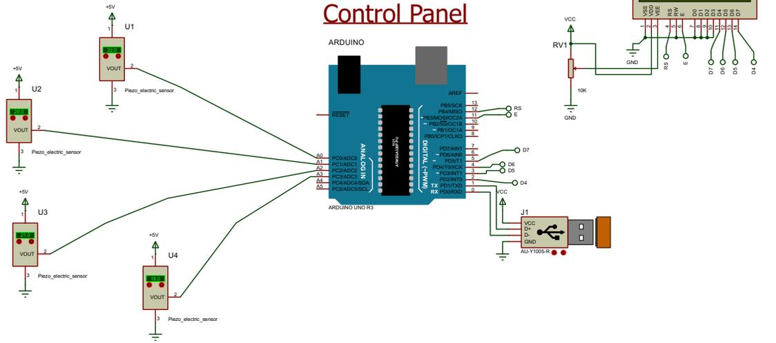
Fig. 4: ARDUINO based sensor module to monitor weight of individual box elements.
