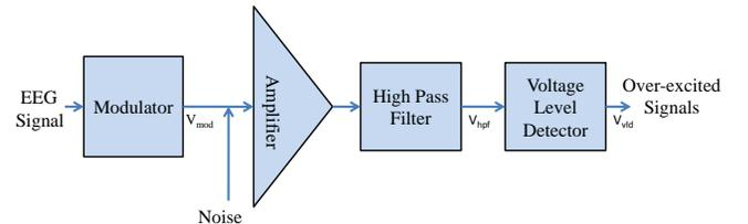
Fig. 3. Proposed hypersynchronous signal detection circuit.
