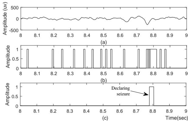
Fig. 6. Transient analysis (a) Zoom inset 8-9 seconds of input EEG signal (b) Output of SRA after first iteration (c) Output of SRA after nth iteration and detection of seizure onset.
