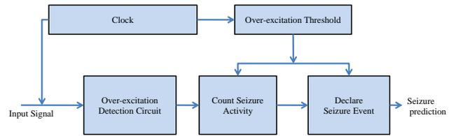
Fig. 2. Proposed architecture of the seizure detector.
