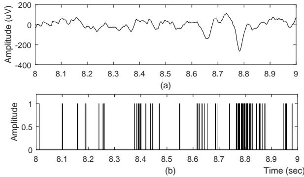
Fig. 5. Transient analysis (a) Zoom inset 8-9 seconds of input EEG signal (b) Output of VLD.
