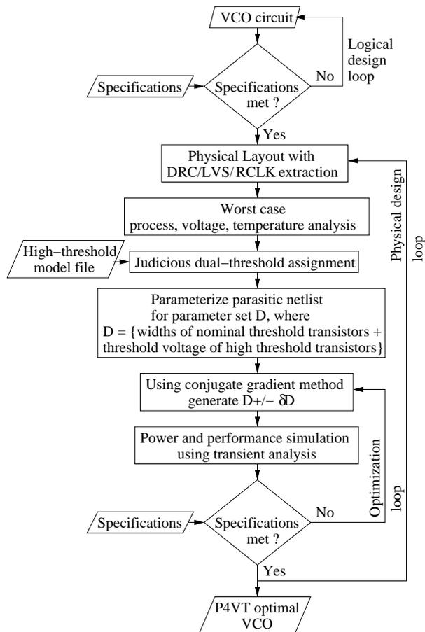
**Figure 1. The P4VT-Optimal Design Flow.**
