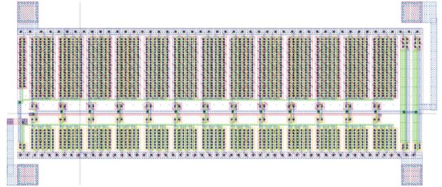
**Figure 5. P4VT-optimal dual- $V_{Th}$  VCO layout.**
