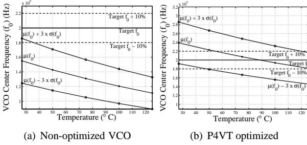
**Figure 2. Center frequency Vs. temperature.**
