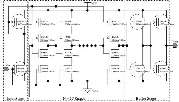
**Figure 4. Candidate transistors for High- $V_{Th}$ .**
