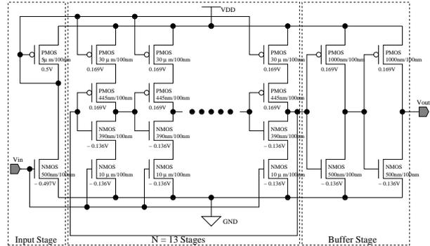
**Figure 6. Parameters of P4VT-optimal VCO.**
