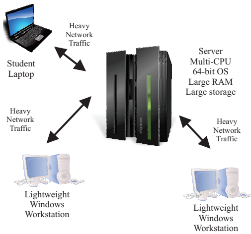
Fig. 1. Client-Server model of lab setup.
