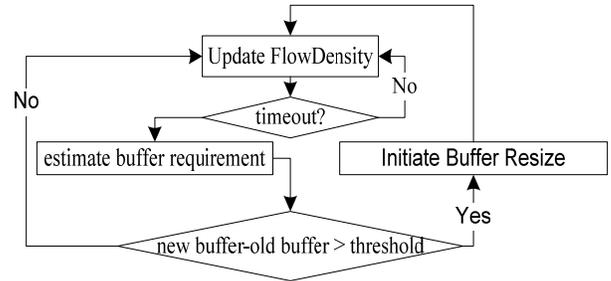
**Figure 7: The Block Level Power Manager FSM**
