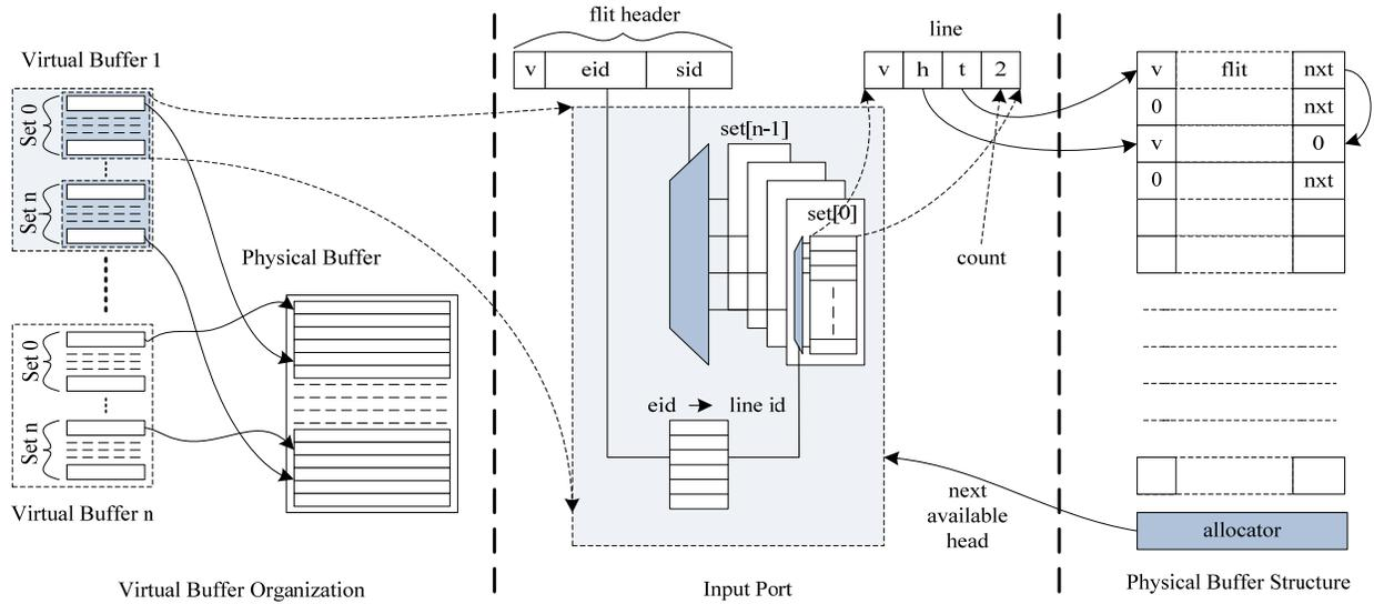
**Figure 5: The Central Buffer Router Architecture**
