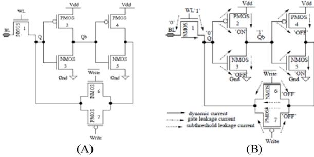
**Figure 3: (A) Single-Ended 7-Transistor SRAM which is tolerant to failures induced by nanoscale process variations. (B) Current paths for write '0' operation of the 7T-SRAM.**
