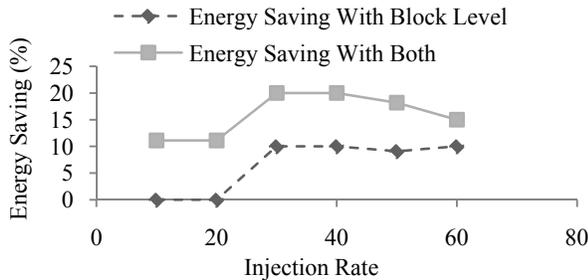
**Figure 12: Energy saving using Dynamic Allocation and Adaptive Flit Inversion over Static Allocation**
