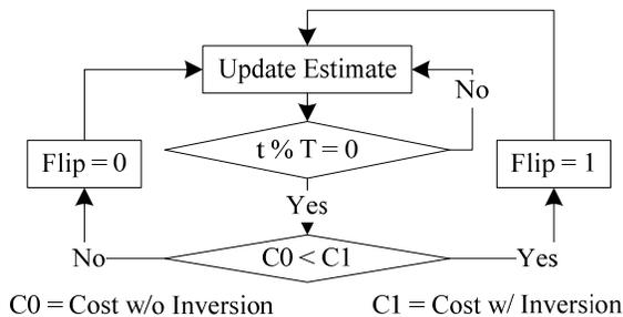
Figure 9: FSM for Dynamic Flit Inversion Controller
