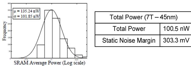
**Figure 4: Total Power Dissipation of 7T SRAM**
