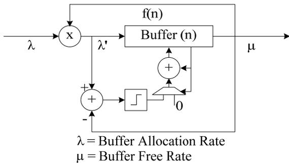
**Figure 6: Block Level Feedback System**
