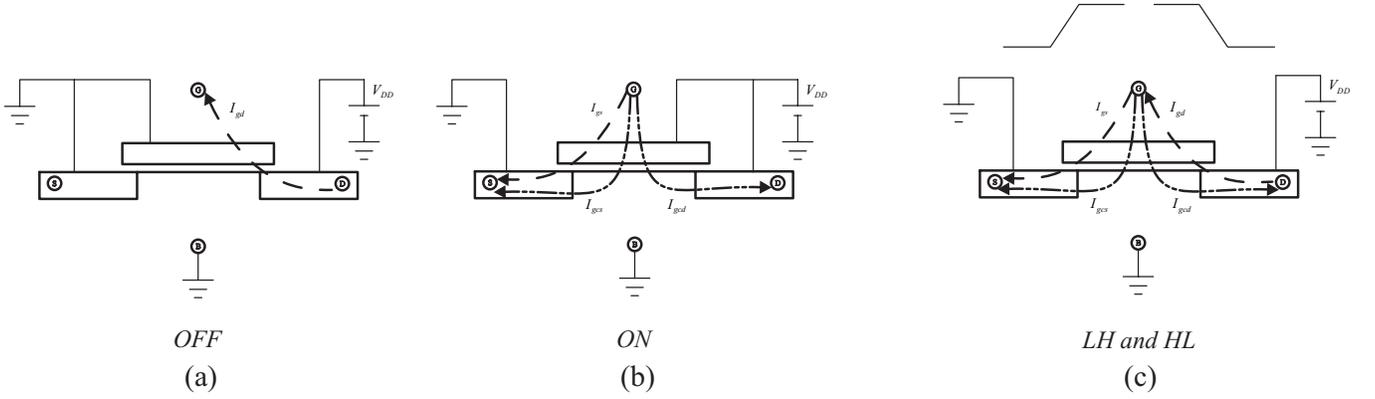
Fig. 3. Gate tunneling current component flow in the various regions of operation of an NMOS.  $I_{gb}$  is negligible and not shown.
