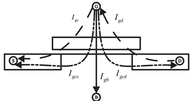
Fig. 1. Gate oxide tunneling current ( $I_{ox}$ ) components in BSIM4.4.0 model.
