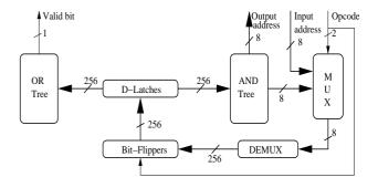
Figure 1: Block Diagram of Our Proposed Hardware Component (For Page Size 4096 bytes and Object Size 16 bytes)
