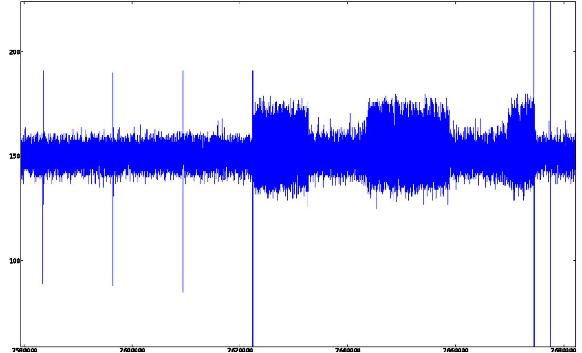
Langer ICR HH 150 probe over Xilinx Spartan3E-1200 FPGA
