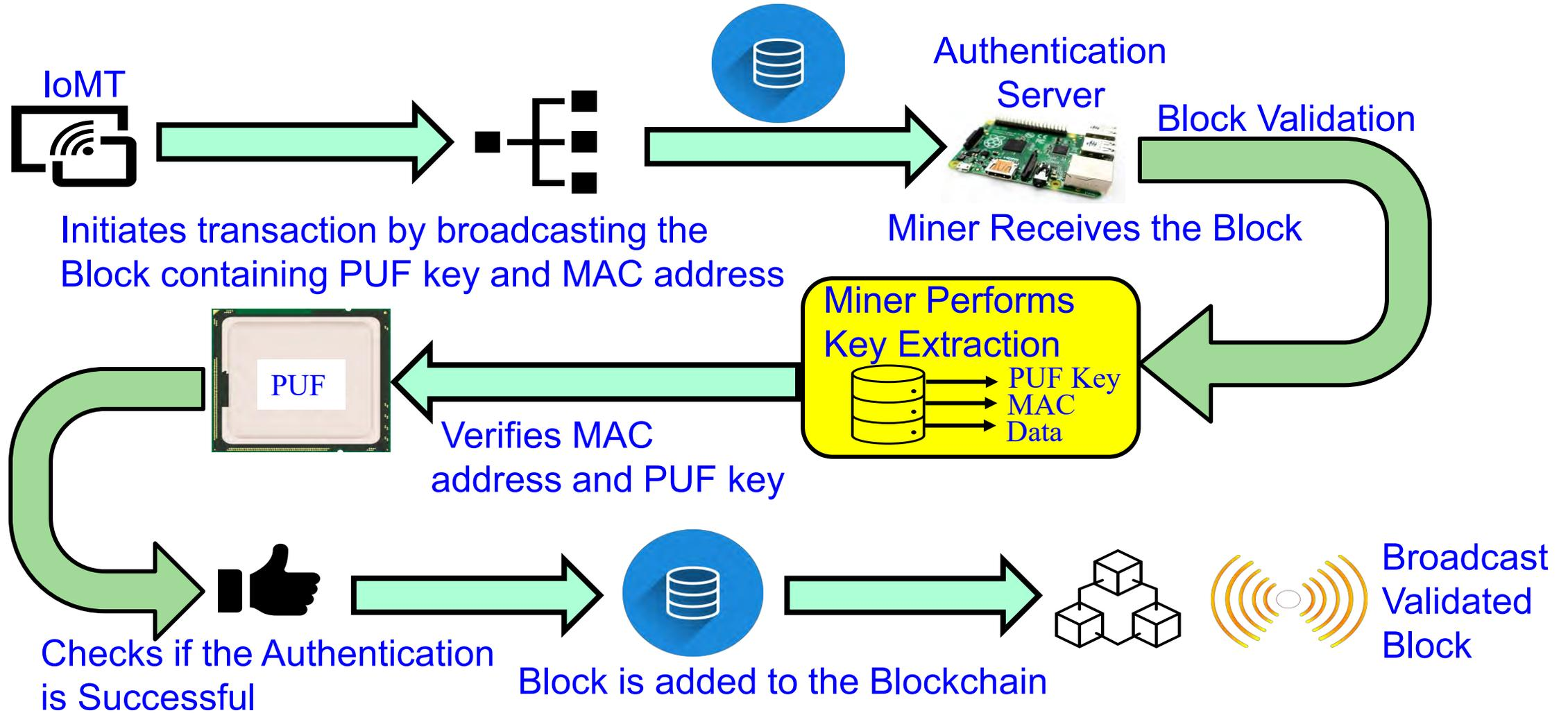
Source: V. K. V. V. Bathalapalli, **S. P. Mohanty**, E. Kougianos, B. K. Baniya, and B. Rout, "PUFchain 2.0: Hardware-Assisted Robust Blockchain for Sustainable Simultaneous Device and Data Security in Smart Healthcare", *Springer Nature Computer Science (SN-CS)*, Vol. 3, No. 5, Sep 2022, Article: 344, 19-pages, DOI: <https://doi.org/10.1007/s42979-022-01238-2>.
