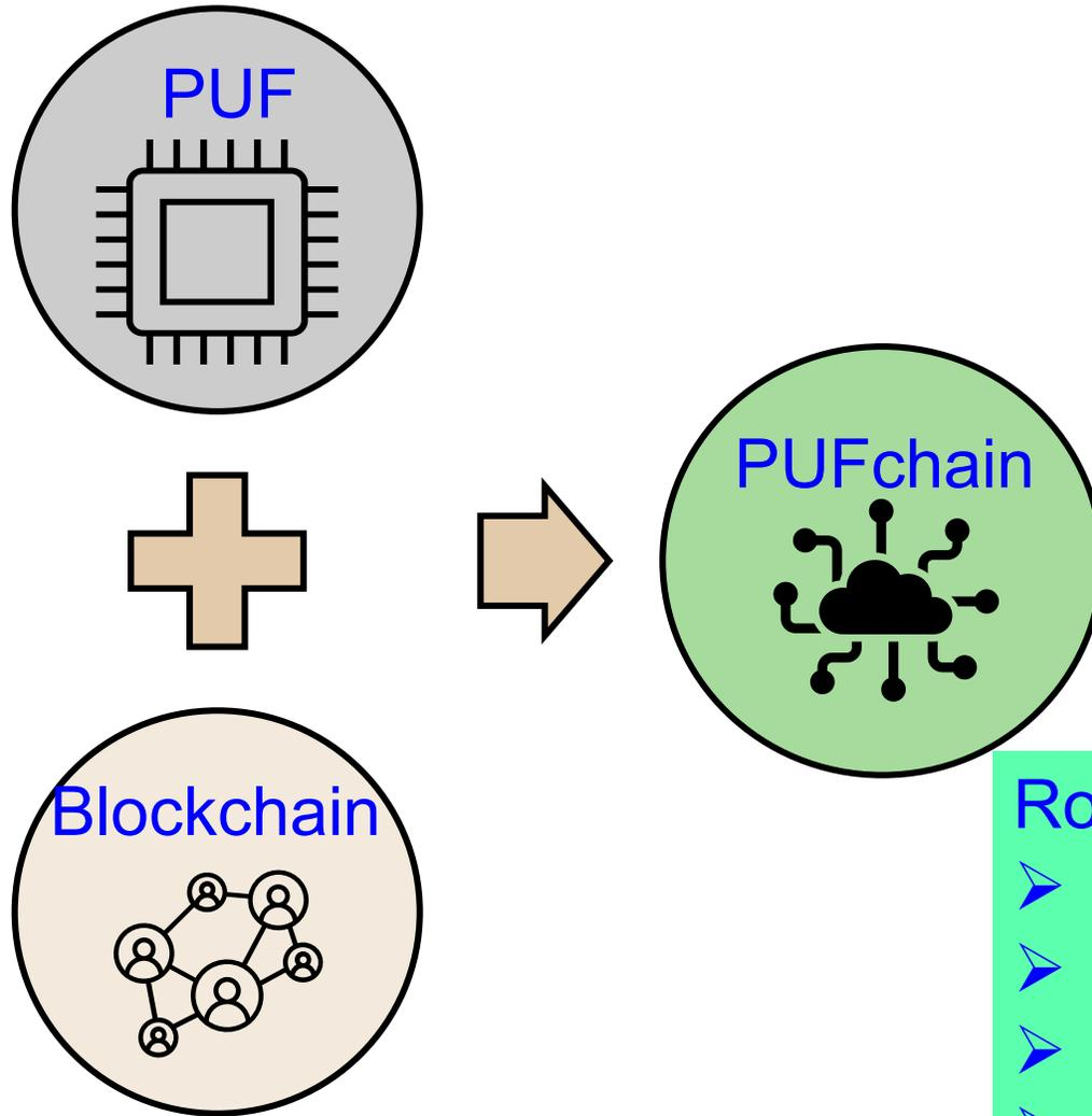
Blockchain Technology is integrated with Physically Unclonable Functions as PUFchain by storing the PUF Key into immutable Blockchain
