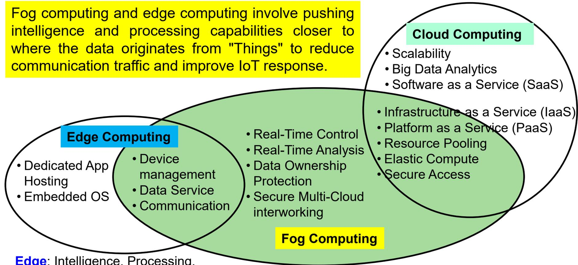
**Edge:** Intelligence, Processing, and Communication - Devices like Programmable Automation Controllers (PACs)
