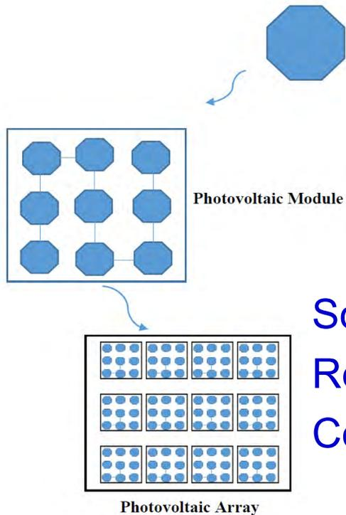
Small solar cells in CE systems to big solar panels in smart grids.
