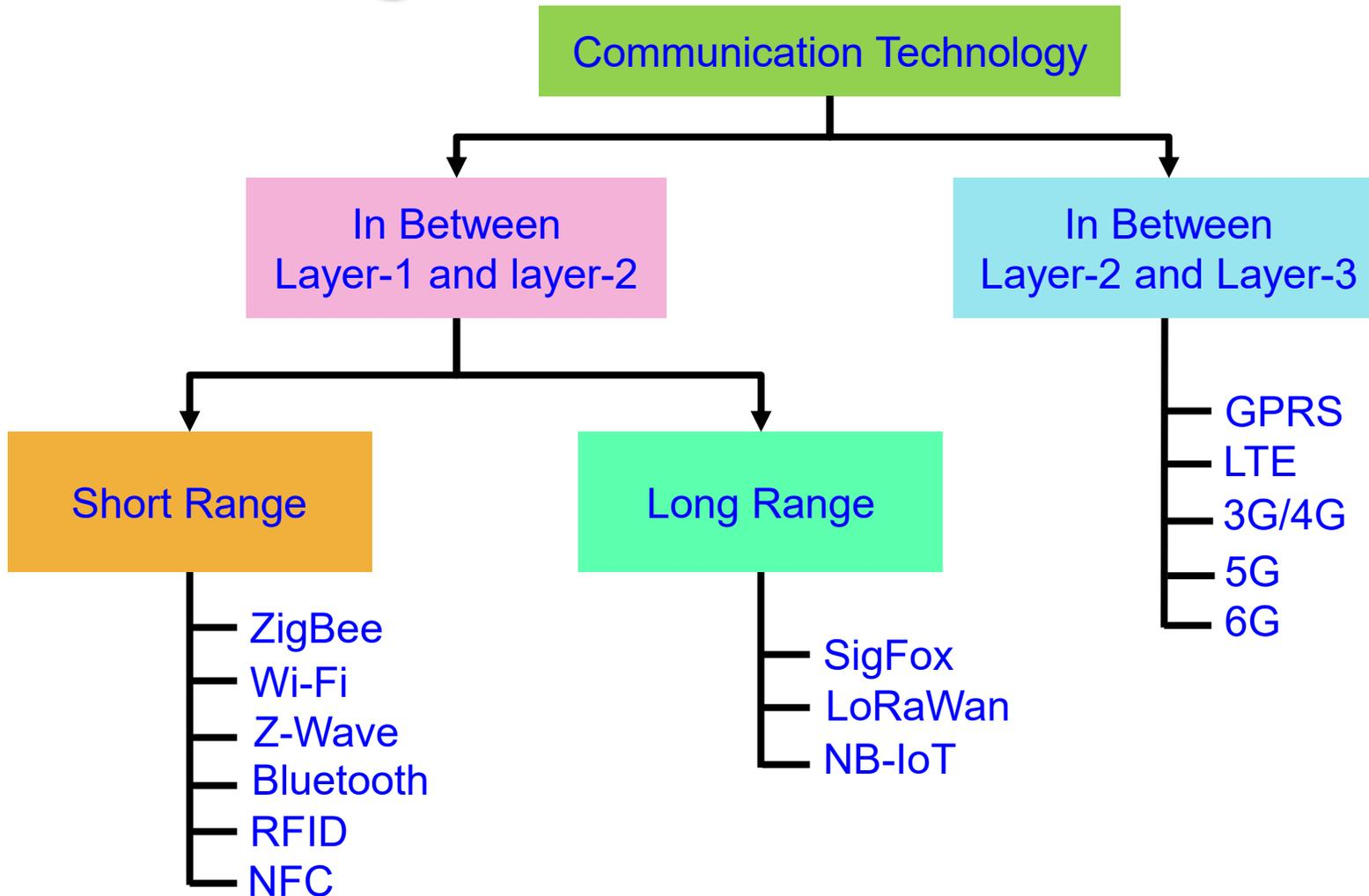
**Connectivity Layer-1** : Near Range ZigBee, Wi-Fi, Z-Wave, Bluetooth, Radio Frequency Identification (RFID), and Near Field Communication (NFC).
