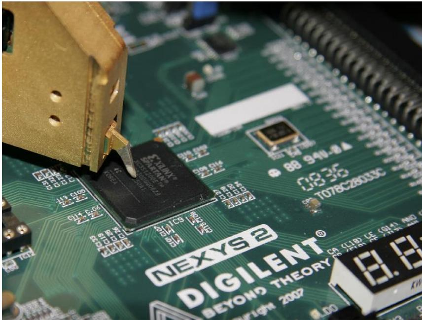
Langer ICR HH 150 probe over Xilinx Spartan3E-1200 FPGA
