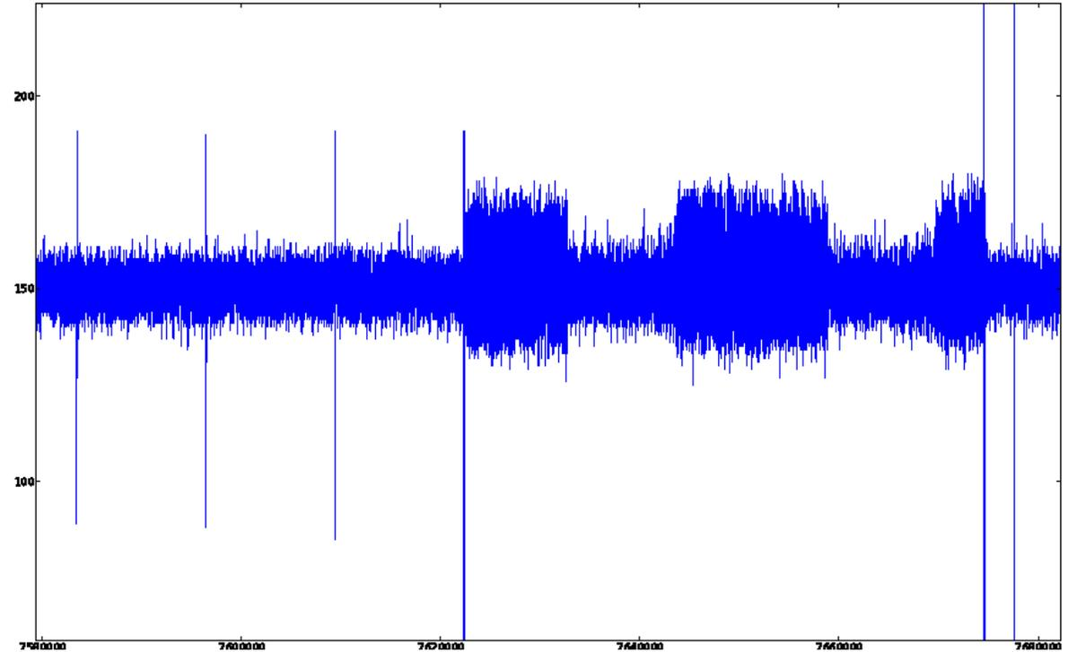
Magnification of the last part of the complete trace. Three trigger signals can be identified: (1) between oscillator phase and error correction phase, (2) between error correction and hashing, and (3) at the end of hashing.
