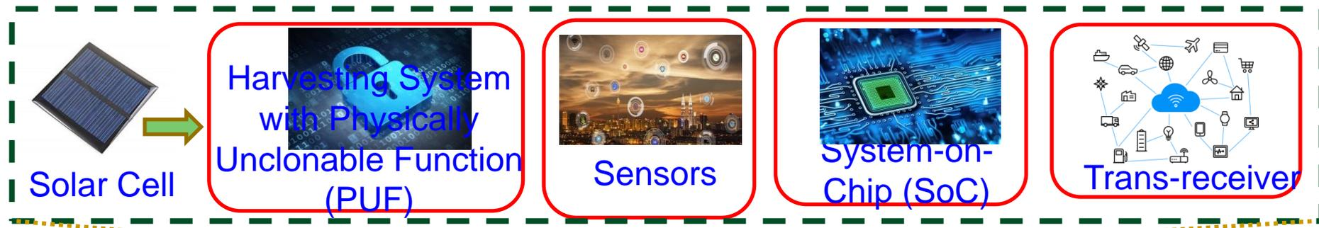
Provides security using PUFs while consuming only  $22 \mu\text{W}$  power due to harvesting.
