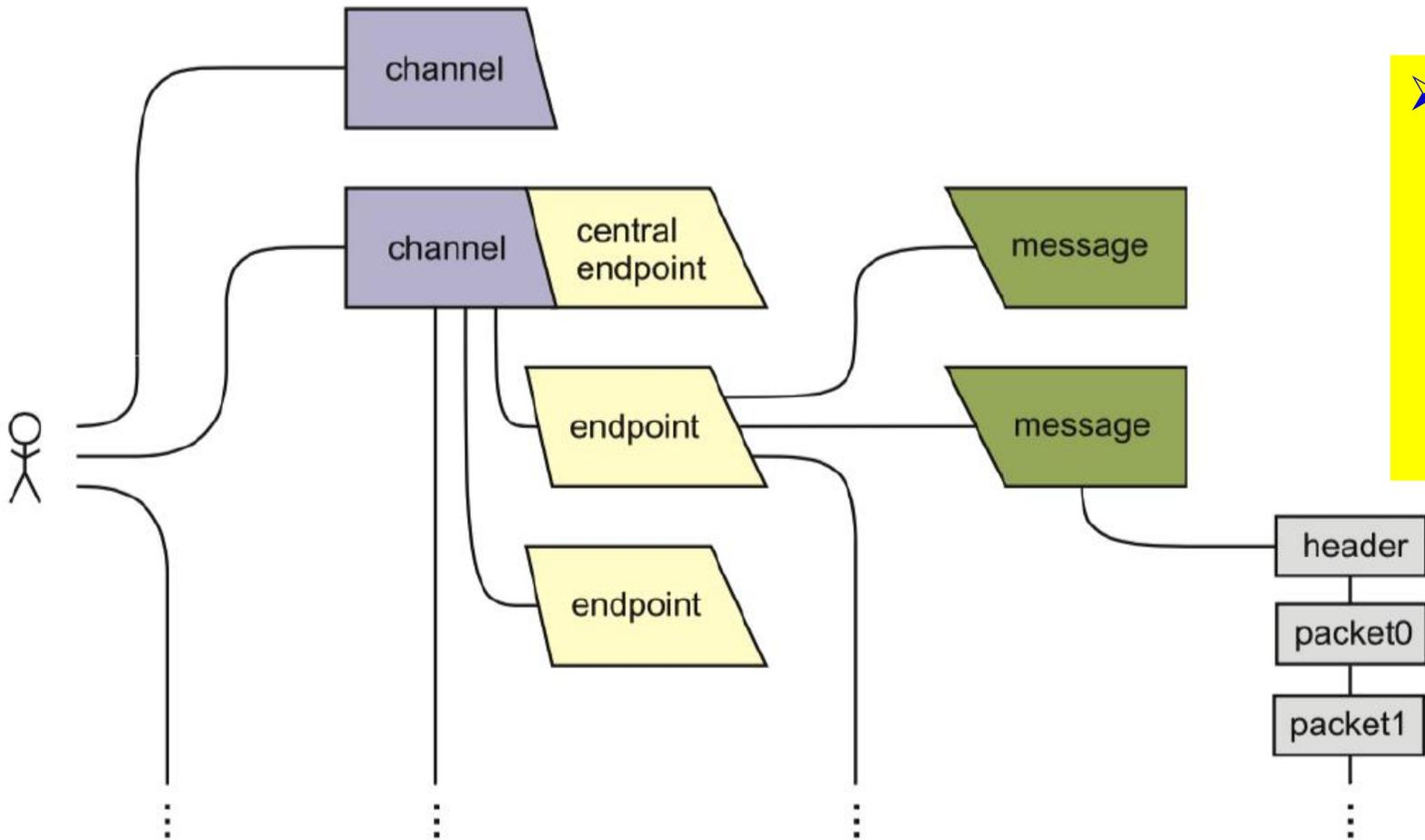
➤ MAM Channel once initiated consists of a sequence of transactions where each transaction provides an address for the next transaction
