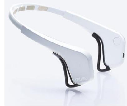
Headband with Embedded Neurosensors
