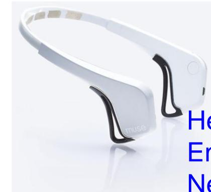
Headband with Embedded Neurosensors
