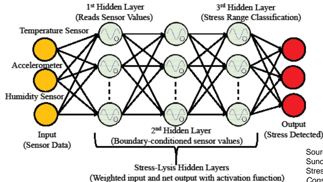
Stress-Lysis - DNN has been trained with a total of 26,000 samples per dataset and has accuracy upto 99.7%.
