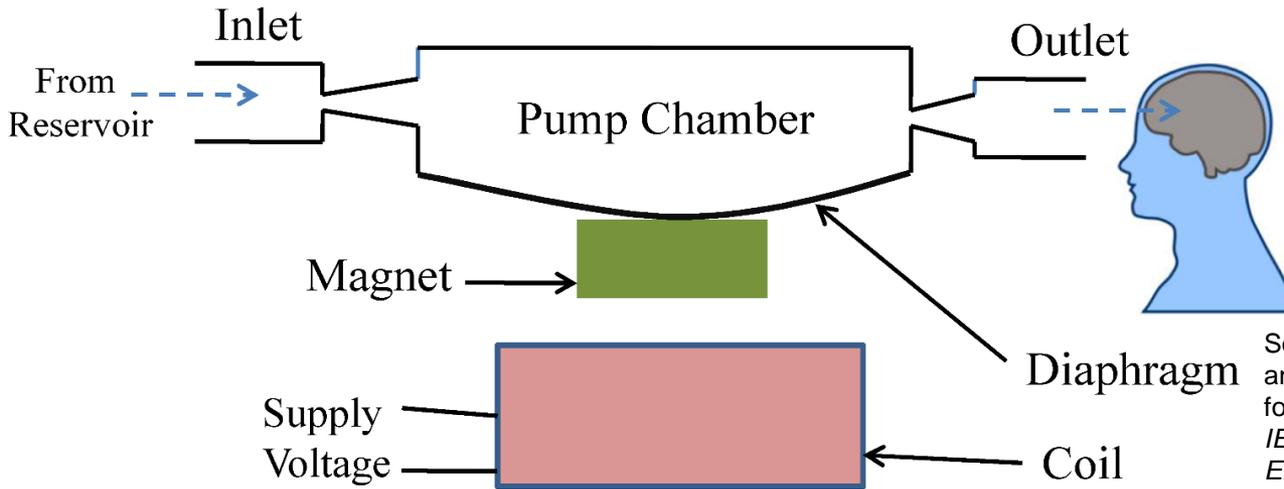
Electromagnetic: Latency – 1.8 Sec, Power – 12.81 mW, Flow Rate – 0.34 mL/min
