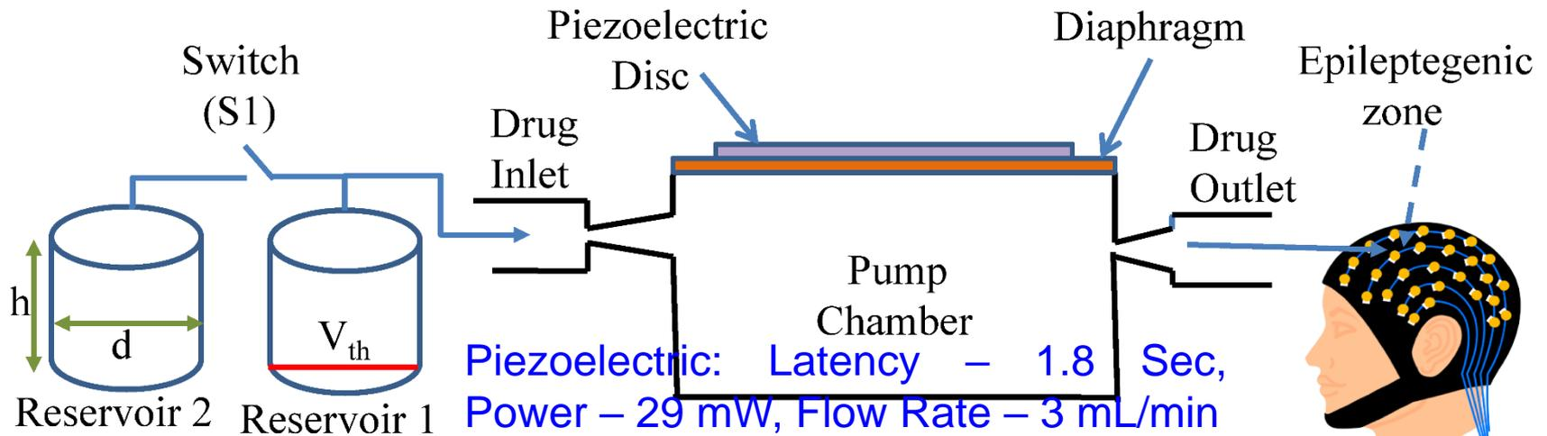
Piezoelectric: Latency – 1.8 Sec, Power – 29 mW, Flow Rate – 3 mL/min
