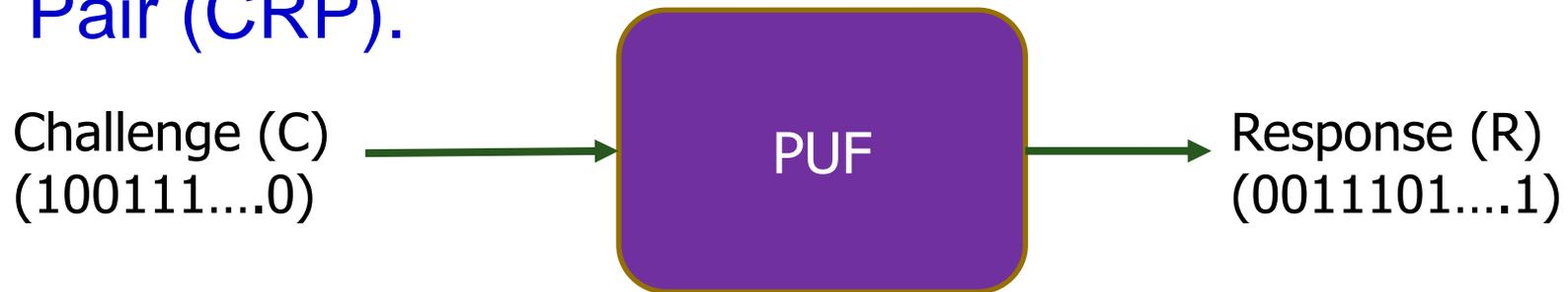
Only an authentic hardware can produce a correct Response for a Challenge.
