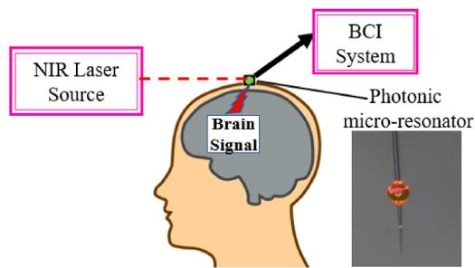
Fig. 1: A BCI system using a photonic micro-resonator.
