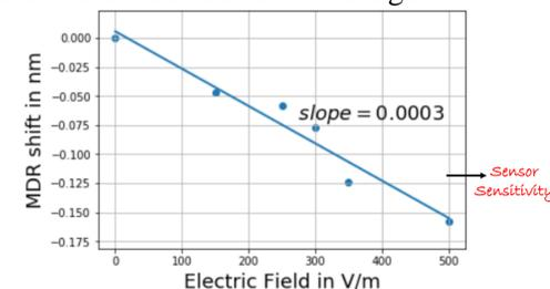
Fig. 10: A plot of MDR shift vs Electric field.
