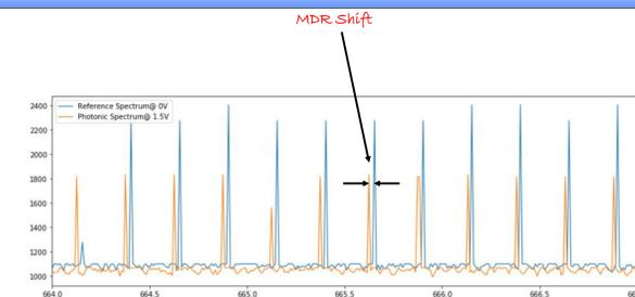
Fig. 8: Spectra at the reference and another voltage
