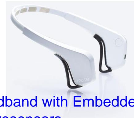
Headband with Embedded Neurosensors
