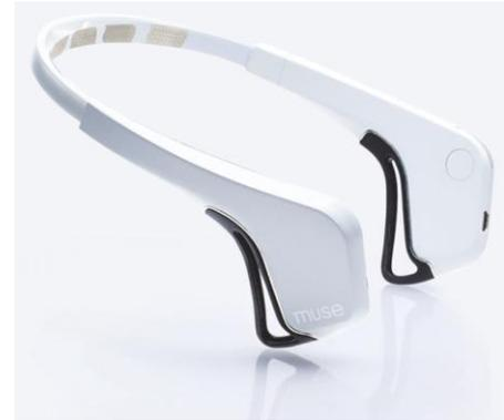
Headband with Embedded Neurosensors
