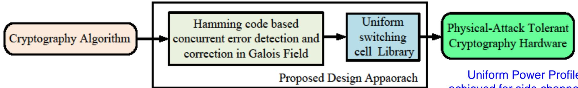
Uniform Power Profile achieved for side channel attack security with some area and minor delay overhead.
