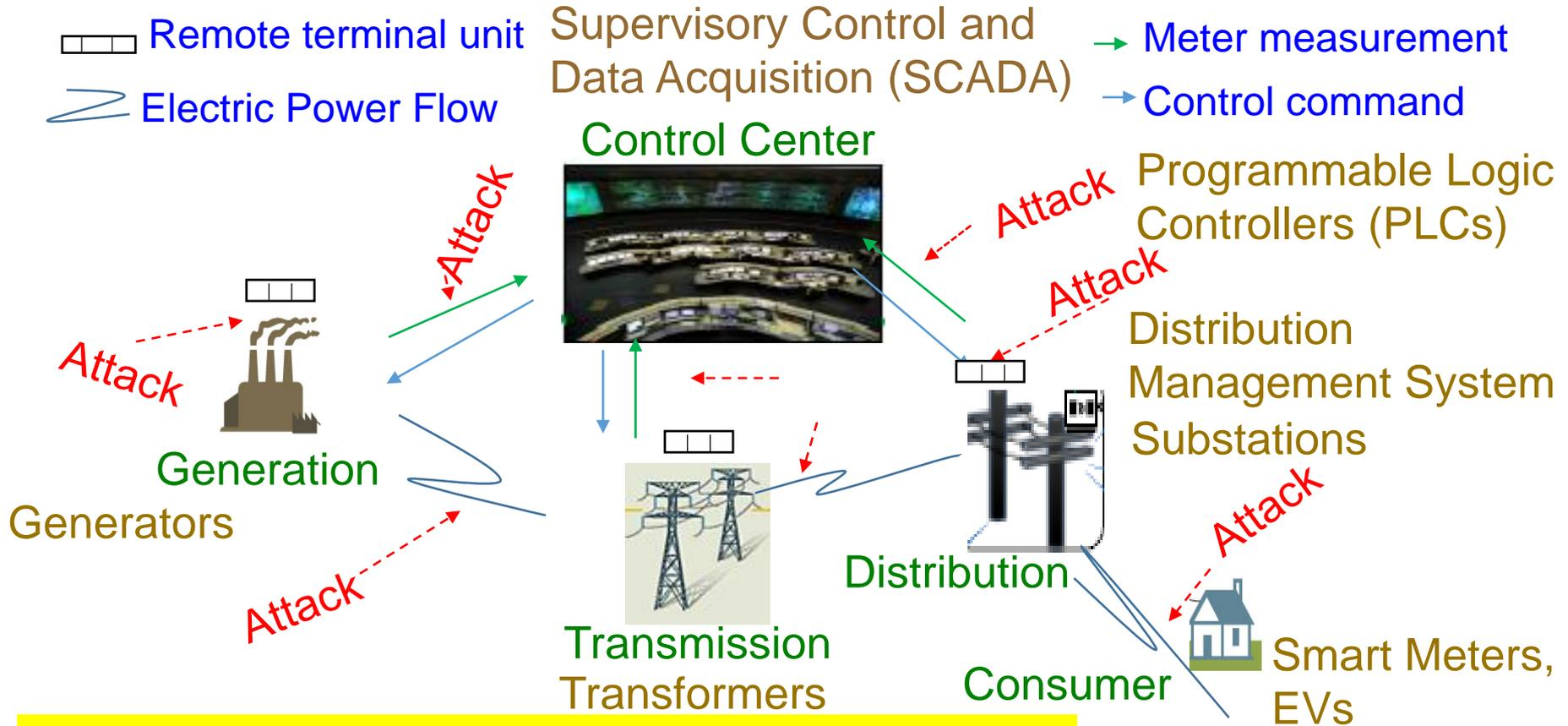
ICT components of smart grid is cyber vulnerable.
