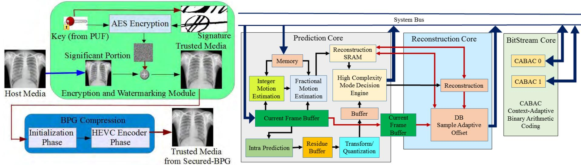
Idea of Secure BPG (SBPG) High-Efficiency Video Coding Architecture
