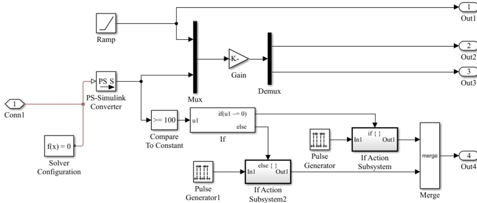
Fig.7: Functional block of the photonic sensor model 2.
