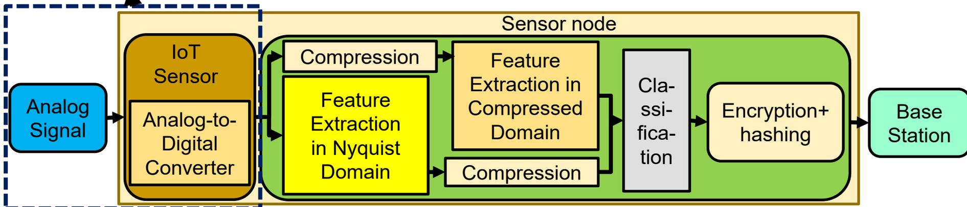
Smart, secure, and energy-efficient IoT sensor architecture
