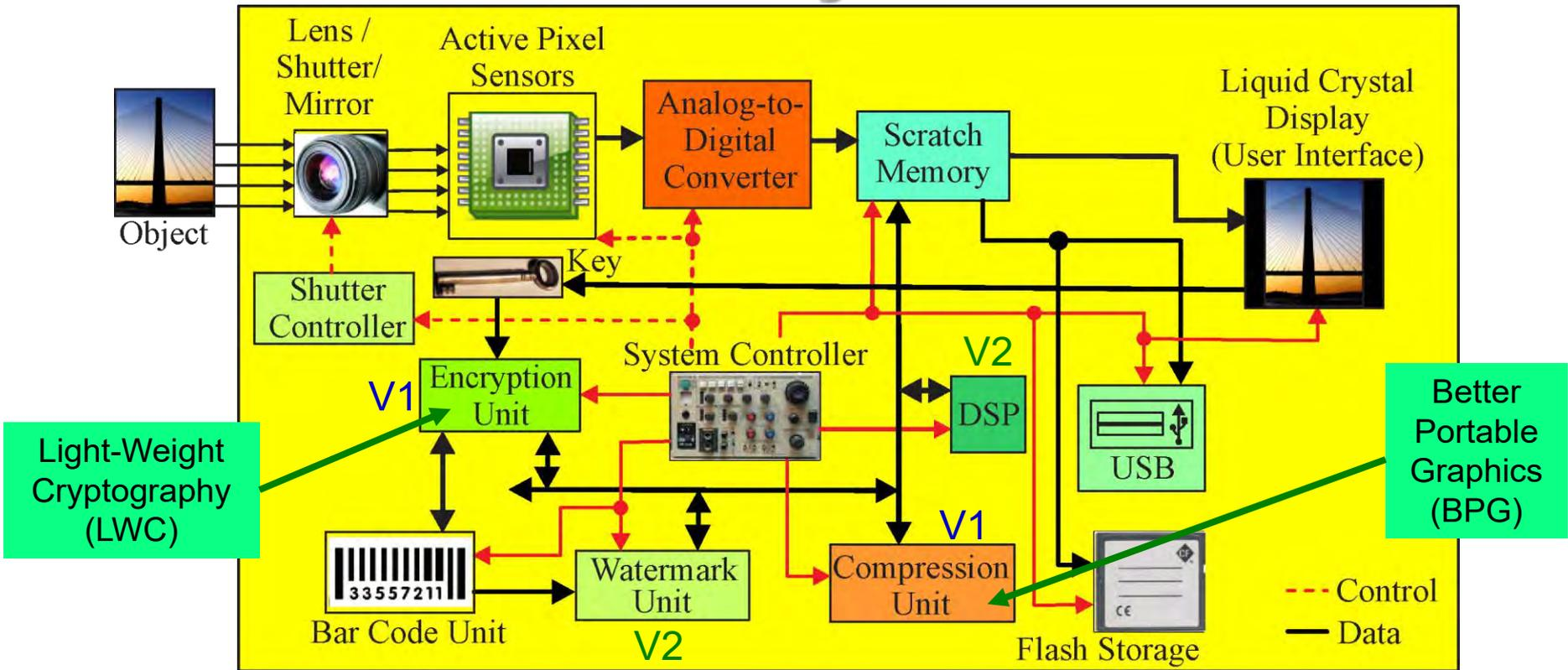
Include additional/alternative hardware/software components and uses DVFS like technology for energy and performance optimization.
