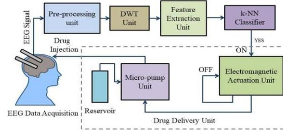
Fig. 2. Architecture of Drug Delivery System ( DDS)
