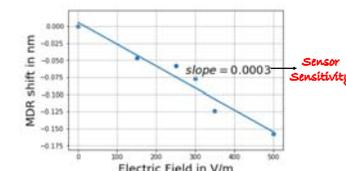
Figure 7: A plot of MDR shift vs Electric field.
