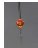
Figure 3: A photonic micro-resonator.
