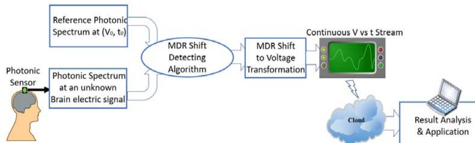
Figure 4: Proposed Photonic Brain-Computer Interface (BCI) Architecture
