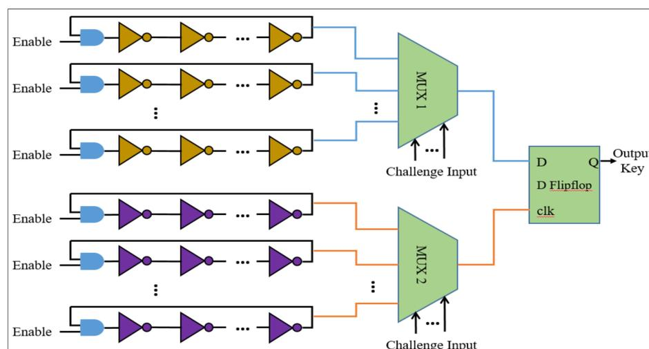
Fig. 2. Hybrid Oscillator Arbiter Physical Unclonable Function
