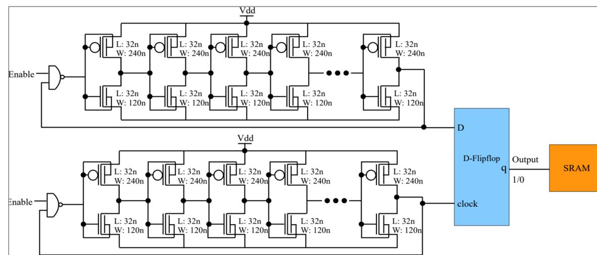
Fig. 3. Circuit Level Representation of Hybrid Oscillator Arbiter PUF
